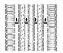
Treadwear indicators are one way to tell when it is time for new tires. Treadwear indicators appear when the tires have only 1.6 mm (1/16 in) or less of tread remaining. See *Tire Inspection*  $\Leftrightarrow$  276 and *Tire Rotation*  $\Leftrightarrow$  276.
