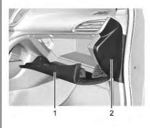
Open the glove box door (1) completely. Grasp the edges of the side instrument panel trim (2) and pull to remove from the instrument panel.
