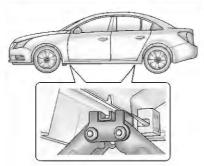
7. Position the jack lift head at the jack location nearest the flat tire. The location is indicated by a notch on the bottom edge of the body side. The jack must not be used in any other position.
