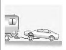
The vehicle can be towed from the front using a dolly. To tow the vehicle using a dolly:
