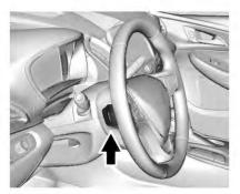
Regen on Demand allows increased deceleration by pressing and holding the steering wheel paddle. It works in D (Drive) and L (Low). The accelerator pedal must be fully released for it to work. The brake pedal must be applied at low speed, because Regen on Demand will not bring the car to a full stop.
