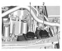
1. High Voltage Battery Coolant Reservoir 2. Power Electronics Coolant Reservoir
