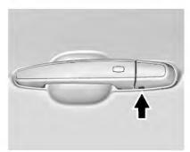
When the Remote Keyless Entry (RKE) transmitter is within 1 m (3 ft) of the driver door, the door can be locked and unlocked by pressing the door handle button. When unlocking from the driver door, the first press will unlock only that door; press again within five seconds to unlock all passenger doors. See *Remote Keyless Entry (RKE) System Operation ⇔ 29.*
