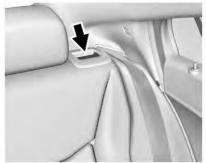
1. Pull the seatback release lever (pictured) to unlock the seatback.
