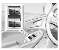
The window switches on the driver door control all windows. Each passenger door has a switch that controls only that window.
