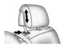
The height of the head restraint can be adjusted. Pull the head restraint up to raise it. Try to move the head restraint to make sure that it is locked in place.
