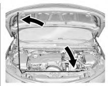
Lift the hood and release the hood prop rod from its retainer above the radiator support. Place the prop rod securely into the slot in the hood.
