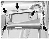
Remove the five screws and pull the entire glove box toward you to release completely. The service door can now be accessed.
