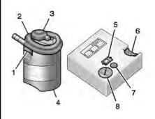
1. Sealant Canister Inlet Valve
