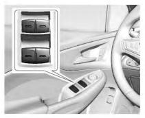
The window switches on the driver door control all windows. Each passenger door has a switch that controls only that window.
