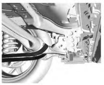
If the car is parked at an angle so that the front toe eye cannot be accessed, wrap a tow strap around both of the rear trailing arms and pull the vehicle onto a flat surface. Do not wrap the tow strap around the rear torque tube.
