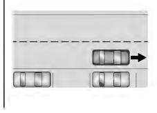
After completely passing a large enough space bordered by two vehicles or other objects, an audible beep occurs and a red symbol displays in the DIC.
