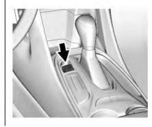
The vehicle has an Electric Parking Brake (EPB). The EPB can always be activated, even if the vehicle is off.
