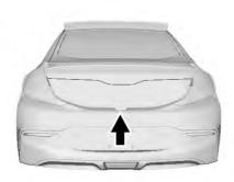
Press on the RKE transmitter to unlock all doors. Press the touch pad on the underside of the hatch and lift.
