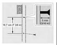
3. Mark and drill the mounting holes in a wall stud or suitable structure. Stay away from any power source.
