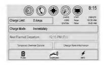
**Immediately :** The vehicle starts charging as soon as it is connected to an electrical outlet. See *Plug-In Charging*  $\Rightarrow$  206.
