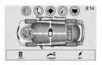
Engine and Regen Power Recovery - Engine is active. Power from the wheels returns to the battery during regenerative braking or coasting.
