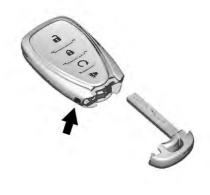
To remove the key, press the button near the bottom of the RKE transmitter, and pull the key out. Never pull the key out without pressing the button.
