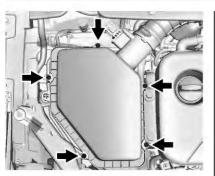
Remove the five screws and lift the air cleaner/filter cover from the air cleaner/filter housing assembly.
