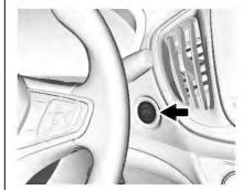
The vehicle has an electronic pushbutton start. The POWER light flashes when the driver door is open and the vehicle is not on. The flashing light will eventually time out. The light is on steady when in ON/ RUN power mode. When the vehicle is turned off, the POWER  $\bigcirc$  light will turn off.
