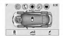
Battery Power - Vehicle is stationary in electric mode and no power is flowing to the wheels.
