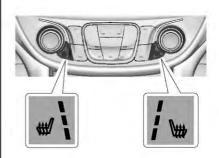
If equipped, the controls are on the center stack. To operate, the vehicle must be on.
