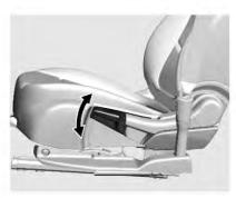
Move the lever up or down to raise or lower the seat.
