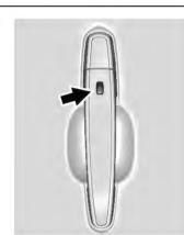
If equipped, the RKE transmitter must be within 1 m (3 ft) of the door being opened. Press the button on the door handle to open. See "Keyless Access Operation" in *Remote Keyless Entry (RKE) System Operation* ⇔ 29.
