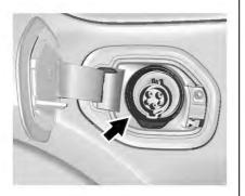
If equipped, the charge port bezel light acts as an additional CSI when the vehicle is plugged in and charging. It will flash along with the CSI on the instrument panel. When the charge port door is open and the vehicle is not plugged in, the bezel light stays on solid to light the charging receptacle.
