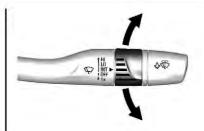
**INT :** Move the lever up to INT for intermittent wipes, then turn the band up for more frequent wipes or down for less frequent wipes.
