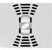
The instrument cluster may have a parking assist display with bars that show "distance to object" and object location information for RPA, and on some vehicles, FPA. As the object gets closer, more bars light up and the bars change color from yellow to amber to red.
