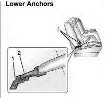
Lower anchors (1) are metal bars built into the vehicle. There are two lower anchors for each LATCH seating position that will accommodate a child restraint with lower attachments (2).
