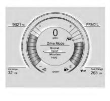
Sport Mode provides more responsive acceleration than Normal Mode, but can reduce efficiency. Use Normal Mode whenever possible.
