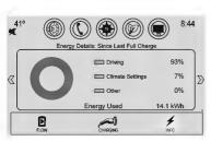
The Energy Details screen displays how energy is being used since the last time the high voltage battery was fully charged. It includes Driving and Accessories, Climate Settings, and Battery Conditioning. The circle graph displays these percentages. The total energy used displays at the bottom of the screen.
