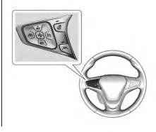
S: Press to turn the cruise control system on and off. A white indicator comes on in the instrument cluster when cruise is turned on.
