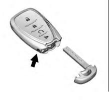
Press the key release button to release the key. The key can be used for all locks.
