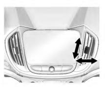
Use the louvers on the air vents to change the direction of the airflow, or to open and close off the airflow.
