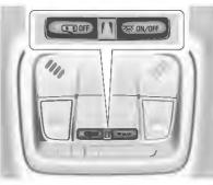
The dome lamp controls are in the overhead console.
