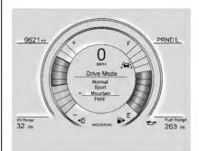
Mountain Mode should be selected at the beginning of a trip before climbing steep, uphill grades and when expecting to drive in very hilly or mountainous terrain. This mode maintains a reserve electrical charge of the high voltage battery to provide better grade climbing performance. While driving in Mountain Mode, the vehicle will have less responsive acceleration.
