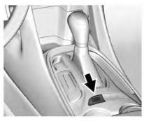
Pressing MODE will display the selectable drive modes in the Driver Information Center (DIC). See *Driver Selected Operating Modes* ⇔ 178 for information on mode operation.
