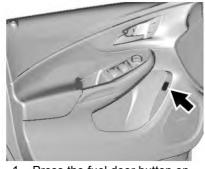
Press the fuel door button on the driver door for one second. A WAIT TO REFUEL message displays on the Driver Information Center.
