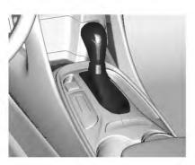
**P**: This position locks the front wheels. It is the best position to use when starting the propulsion system because the vehicle cannot move easily.
