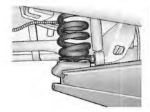
When lifting the vehicle from the rear, place the service jack directly under the spring seat.
