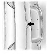
RKE transmitter must be within 1 m See Remote Keyless Entry (RKE) hatch with the vehicle locked, the (3 ft). Press the touch pad on the underside of the hatch and lift up. Keyless Access: To open the System Operation on page 2-2.
