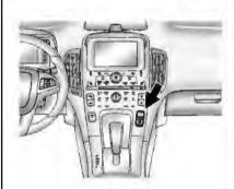
The vehicle has an Electric Parking Brake (EPB). The switch is on the center stack. The EPB can always be activated, even if the vehicle is off. To prevent draining the 12-volt battery, avoid repeated cycles of the EPB system when the vehicle is off.
