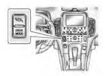
Press the DRIVE MODE button to display selectable drive modes in the Driver Information Center (DIC). Continue pressing to scroll through the modes.
