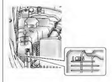
Fill the coolant surge tank with the proper mixture to the cold fill line.
