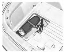
Open the rear hatch, lift the load support floor covering, and remove the charge cord. It is near the tire sealant and compressor kit. Pull up on the charge cord handle. The vehicle plug is stored as shown. 4. Plug the charge cord into the electrical outlet. See *Electrical Requirements for Battery Charging on page 9-51*. Verify the charge cord status. See *Charge Cord on page 9-50* and the charge cord user guide.
