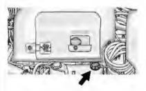
Check to see if coolant is visible in the reservoir. If coolant is visible but the coolant level is below the cold fill line, there could be a leak in the cooling system.
