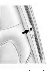
off, the CSI indicates the following: plugged in and the vehicle power is windshield. When the vehicle is instrument panel near the Indicator (CSI) at the center of the The vehicle has a Charging Status
