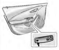
The rear door safety locks prevent passengers from opening the rear doors from inside the vehicle.
