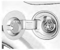
Plug in the vehicle plug of the charge cord into the charge port on the vehicle. Verify that the charging status indicator illuminates on top of the instrument panel and a horn chirp occurs. See Charging Status Feedback on page 9-47. 6. To arm the charge cord theft alert, lock the vehicle with the RKE transmitter. To disable this feature, see "Charge Cord Theft Alert" in Vehicle Personalization on page 5-50.
