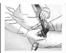
If the webbing locks in the latch plate before it reaches the buckle, tilt the latch plate to flat to unlock.
