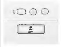
The button for TCS and StabiliTrak is on the overhead console.
