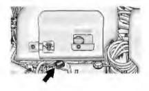
Check to see if coolant is visible in the high voltage battery coolant reservoir. If coolant is visible but the coolant level is below the cold fill line, there could be a leak in the cooling system.
