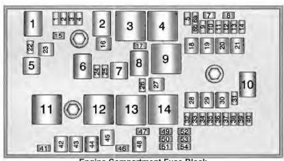
**Engine Compartment Fuse Block**
