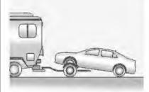
The vehicle can be towed from the front using a dolly. To tow the vehicle using a dolly:
