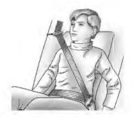
Buckle and position the safety belt as described previously in this section. Make sure that the shoulder belt crosses the shoulder To remove and store the comfort guide, squeeze the belt edges together so that the safety belt can be removed from the guide. Slide the guide back into its storage clip located on the interior body trim next to the side of the seatback.
