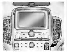
The power door lock switches are on the center stack.
