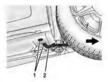
Place the tow chain hooks (2) into one of the torque box openings (1) behind the front wheels.
