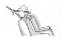
If the rear outboard seating position you are using has an adjustable head restraint and you are using a dual tether, route the tether around the head restraint.
