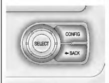
**CONFIG:** Press to select either the Simple or Enhanced instrument cluster configuration display.
