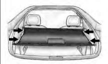
There is a cover for the rear cargo area. Use the four cargo cover loops to hook the cover to the side panels.
