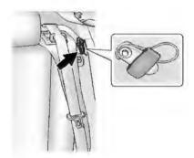
Remove the guide from its storage clip on the interior body trim next to the rear seat.
