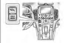
To view the Power Flow, Charging, and Energy Information, press the button on the center stack.
