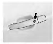
When the Remote Keyless Entry (RKE) transmitter is within 1 m (3 ft) of the driver door, the door can be locked and unlocked by pressing
