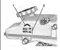
With the vehicle not running for at least one minute, the maximum fluid level (1) is at the top of the reservoir body. With the vehicle running, the fluid level should be in the proper operating range (2) between the MIN and MAX marks. If it is not, have the brake hydraulic system checked to see if there is a leak.
