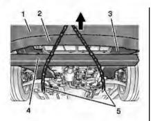
4. Place a 1.2 m (4 ft) X 102 mm (4 in) X 102 mm (4 in) wood beam (4) under the front cradle crossmember (3), and on top of both tow chains (5) to ensure the tow chains do not come into contact with the front fascia (1).
