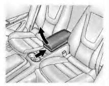
To remove the armrest storage bin, press the button and lift the armrest storage bin up.
