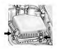
2. Remove the air cleaner cover. See Engine Air Cleaner/Filter on page 10-13.  Remove the air cleaner assembly by pulling up to release the rear two retention posts from the securing grommets. Then pull it forward to remove the remaining retention post from the securing grommet.
