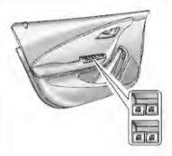
The window switches on the driver door control all windows in the vehicle. Each passenger door has a switch that controls only that window.
