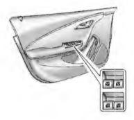
The power window switches are on the driver door armrest. Each passenger door has a switch that controls only that window.
