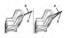
A top tether (3, 4) anchors the top of the child restraint to the vehicle. A top tether anchor is built into the vehicle. The top tether attachment (2) on the child restraint connects to the top tether anchor in the vehicle in order to reduce the forward movement and rotation of the child restraint during driving or in a crash.
