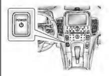
The vehicle has an electronic pushbutton start. The POWER  $\circlearrowleft$  button light flashes when the driver door is open and the vehicle is not
