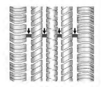
Treadwear indicators are one way to tell when it is time for new tires. Treadwear indicators appear when the tires have only 1.6 mm (1/16 in) or less of tread remaining. See *Tire Inspection on page 10-53* and *Tire Rotation on page 10-53*.
