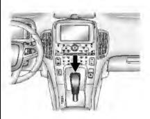
**P (Park):** This position locks the front wheels. It is the best position to use when starting the propulsion system because the vehicle cannot move easily.
