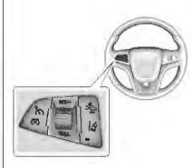
n (On/Off): Press to turn the cruise control system on and off. A white indicator comes on in the instrument cluster when cruise is turned on.
