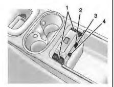
In the armrest storage area there is an auxiliary jack (2), USB port (3), and accessory power outlet (4). Cords from accessories can be routed through the openings (1) on each side. See *Power Outlets on page 5-7* and "Audio Players" in the infotainment manual.
