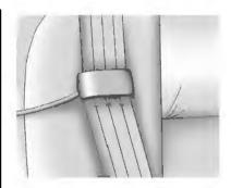
3. The belt should not be twisted and it should lie flat. The elastic cord must be under the belt and the guide on top.
