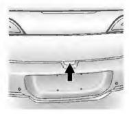
**Keyless Access:** To open the hatch with the vehicle locked, the RKE transmitter must be within 1 m (3 ft). Press the touch pad on the underside of the hatch and lift up. See *Remote Keyless Entry (RKE) System Operation on page 2-2.*
