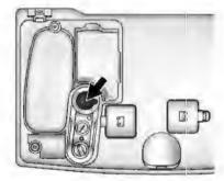
Remove the tire sealant and compressor kit.
