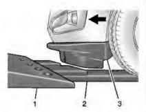
Ramps (2) are required for the front fascia (3) to clear the flatbed (1). The ramp height should be approximately 102 mm (4 in). Lower the flatbed onto the set of ramps.
