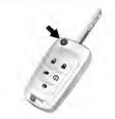
Press the key release button to extend the key. The key can be used for all locks.
